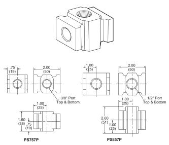
A Modular Manifold Block can be used between any two Modular units to give additional outlet ports. The Manifold Block provides 2 additional outlets in 3/8" and 1/2" sizes. Any standard pipe plug can be used to close off unused ports.
