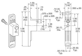
Wall Mounting Kits are available for mounting your Modular Assemblies and can be assembled and used with any standard body connector set.
