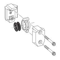
Body Connectors allow you to easily assemble and disassemble Modular Combinations.
