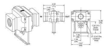
Lockout Valves provide positive shut-off and exhaust capability to isolate Modular units so they can be easily removed from the line and can be locked in a closed position. Center position can be used as a slow start. Accepts #3 padlock.
